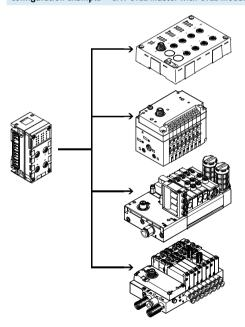
The CPX-CTEL master provides 4 external I-Port interfaces, each of which can be connected with a device. I-Port is an interface for exchanging serial data for connecting decentralised modules or valve terminals from Festo. The I-Port interface is based on IO-Link and is compatible with it in certain areas. The connection type corresponds to a star topology. In other words, only one module or valve terminal can be connected to each I-Port.
